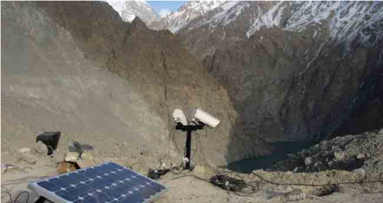
The monitoring station, high above the lake at Attaabad, keeping a watchful eye on the water level
